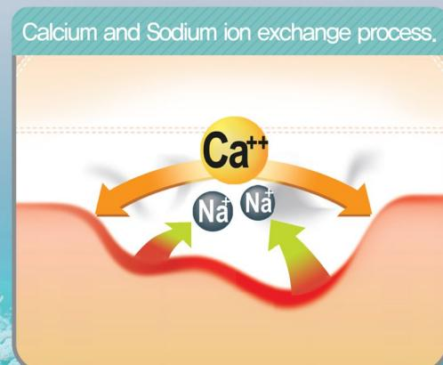
Calcium and Sodium ion exchange process.
